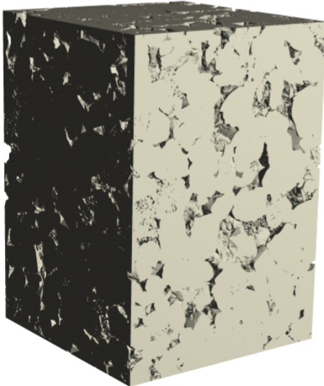
Berea Sandstone modeled from imported 3D data using ImportGeo-Vol
